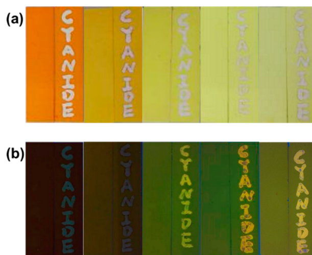
Figure 10. Color changes on the silica gel plates (a) under visible-light and (b) under UV light at 365 nm from left to right are PY, PY-CN, AN, AN-CN, NA, NA-CN, B1, B1-CN, B2, and B2-CN.
